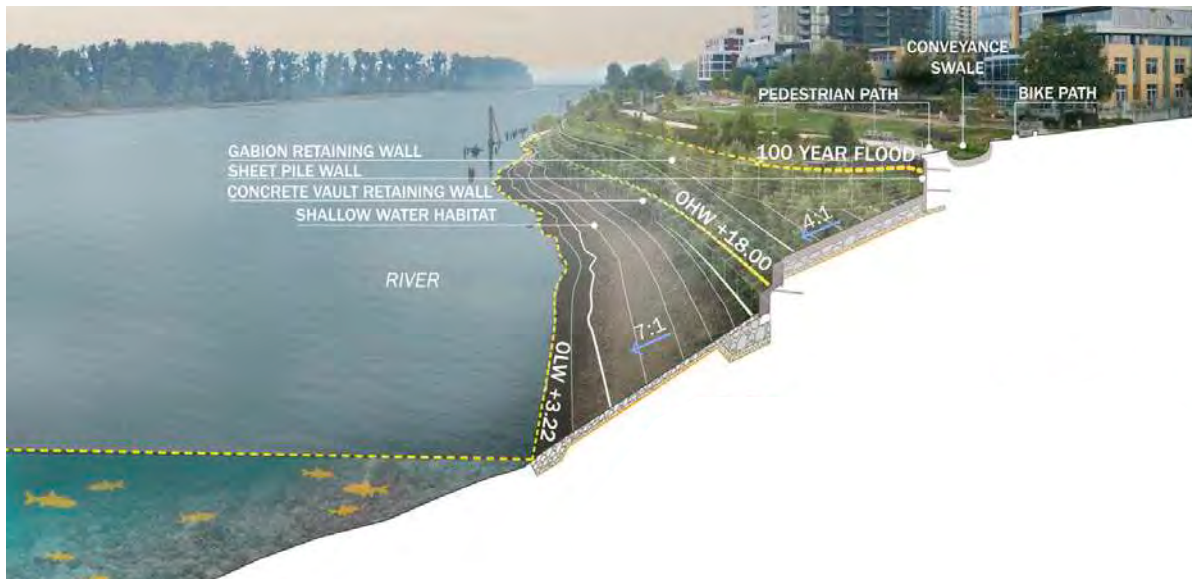
Example of nature based solutions, including a combination of habitat and human-made infrastructure in flood protection. (Portland, OR)
